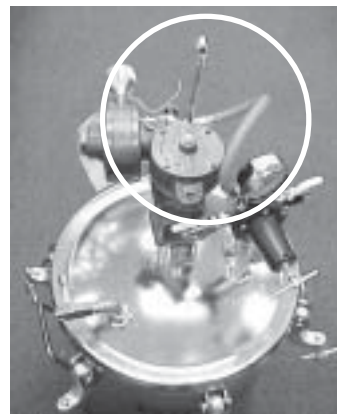
Assemble hose to either manifold using a 5/8 wrench.
