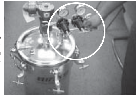
Assemble double regulator to manifold using an 11/16 wrench.
